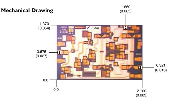
Units: millimeters (inches) Bond pad dimensions are shown to center of bond pad. Thickness: 0.110 +/- 0.010 (0.0043 +/- 0.0004), Backside is ground, Bond Pad/Backside Metallization: Gold All Bond Pads are 0.100 x 0.100 (0.004 x 0.004). Bond pad centers are approximately 0.109 (0.004) from the edge of the chip. Dicing tolerance: +/- 0.005 (+/- 0.0002). Approximate weight: 1.784 mg.
